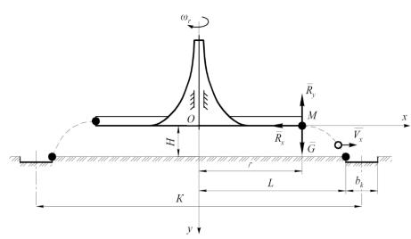
Figure 3. The equivalent diagram for the flight of a particle with the mass of *M*, as thrown from the disc-type tool when spreading mineral fertilisers.
