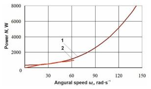
**Figure 5.** The dependence of the power demand *N* when driving the centrifugal tool for spreading mineral fertiliser in terms of the angular speed  $\omega_{r}$ : 1) theoretical and 2) experimental dependence
