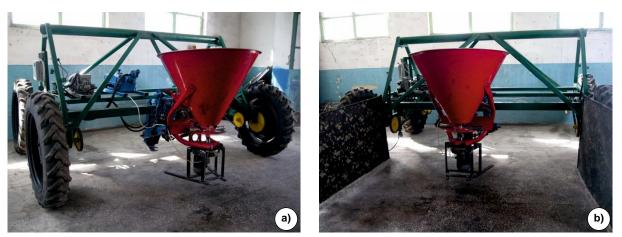
Figure 1. Agricultural gantry while conducting experimental studies, with a mineral fertiliser spreader installed at the front: a) general view; b) view with protective screens installed on both sides
