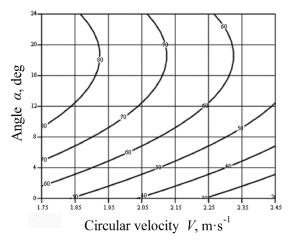
**Figure 4.** Two-dimensional section of response surface of relation between separation intensity  $I_S$  on the one hand and separator inclination angle  $\alpha$  and circular velocity *V* of cleaning spiral rotation on the other hand.
