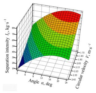
**Figure 3.** Response surface of relation between separation intensity  $I_s$  on the one hand and separator inclination angle  $\alpha$  and circular velocity *V* of cleaning spiral rotation on the other hand.
