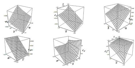
**Figure 2.** Graphs of the normal strain rate components of the soil  $\dot{\epsilon}_{xl}$ ,  $\dot{\epsilon}_{yl}$ ,  $\dot{\epsilon}_{zl}$ , depending on the coefficients *a*, *b*, *c* of the equation of the plane
