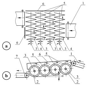
**Figure 1.** Design layout of spiral-type potato cleaning device: a – top view; b – side view: 1 – feeding elevator; 2 – spirals of cleaning rolls; 3 – shafts actuating rotary motion of spirals; 4 – hubs; 5 – free ends of spirals; 6 – screens; 7 – discharge elevator;  $\alpha$  – inclination angle
