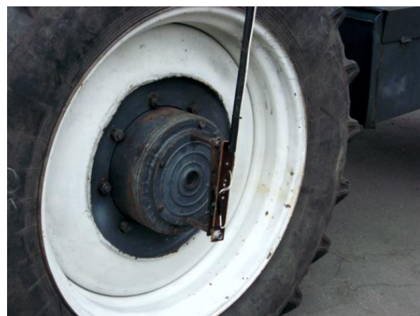
Figure 6. Wheel rpm pickup
