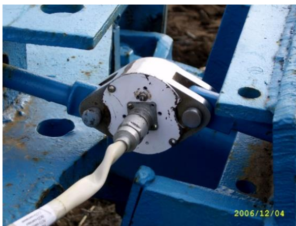
Figure 5. Draught strain-gauge link
