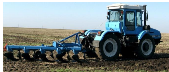
Figure 4. Ploughing implement on HTZ-17221 carrying tractor
