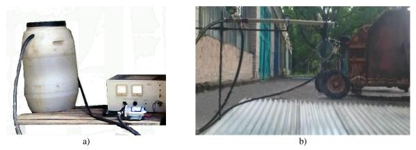
Figure 4. A general view of the experimental setup and the spraying process: a) pumping device and adjuster; b) customized laboratory equipment.
