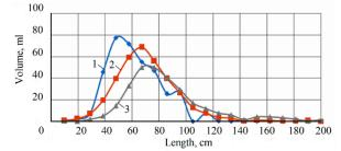
**Figure 6.** Distribution of the sprayed liquid over the corrugated surface at a speed of the lateral airflow of 0–6 m s<sup>-1</sup> and air pressure in the pneumatic system to 0.15 MPa: 1 - V = 0 m s<sup>-1</sup>; 2 - V = 3 m s<sup>-1</sup>; 3 - V = 6 m s<sup>-1</sup>
