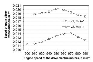
**Figure 6.** Dependence of the speed of grain vibro-transportation on the engine speed of the drive electric motors: 1 - speed of vibro-transportion under eccentricity of imbalances e = 0.025 m; 2 - speed of vibro-transportion under eccentricity of imbalances e = 0,015 m.
