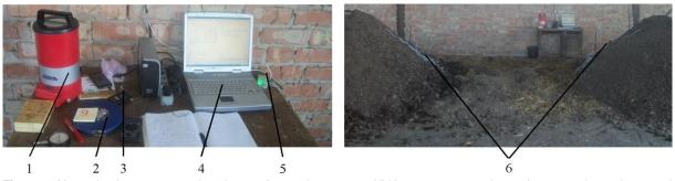
**Figure 3.** Measuring instruments and equipment (1 – moisture meter VLK-01; 2 – construction roulette; 3 – electronic manual scales; 4 – personal computer; 5 – electronic thermometer TM-32/H-5T; 6 – DS18B20 temperature sensors)
