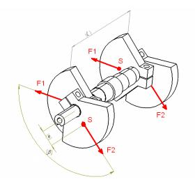
Figure 4. The layout of imbalances on the drive shaft
