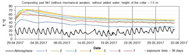
Figure 10. Dynamics of the temperature field of the composting pad №1
