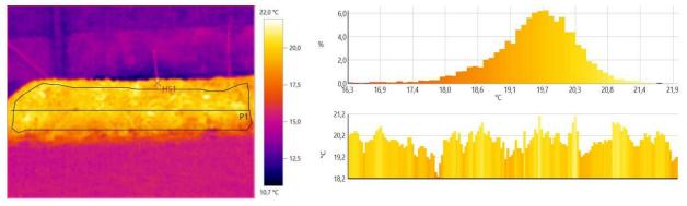
Figure 15. Static temperature field of the surface of the composting pad №2 (composting pad height of 1.0 m without further mechanical aeration and additional humidification)
