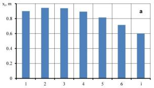
Figure 7. Distribution of distance between the holes (a) and air velocities through them (b) along the length of the air duct of the contaminated air intake ventilation system
