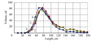
**Figure 7.** Distribution of the liquid over the corrugated surface depending on the air pressure in the pneumatic system 0–0.15 MPa at speed of a lateral air stream of 6 m s<sup>-1</sup>:  $1 - P_p = 0$  MPa;  $2 - P_p = 0.05$  MPa;  $3 - P_p = 0.10$  MPa;  $3 - P_p = 0.15$  Mpa
