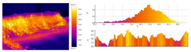
Figure 19. Static temperature field of the longitudinal section of the composting pad №4 (composting pad 1.5 m high with subsequent mechanical aeration and with additional humidification)
