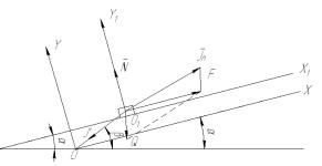
Figure 5. Scheme of action of forces on a particle of bulk material, which is placed on a vibrating tray
