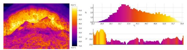
Figure 18. Static temperature field of the cross-section of the composting pad №3 (composting pad 1.5 m high with subsequent mechanical aerations and with additional humidification)
