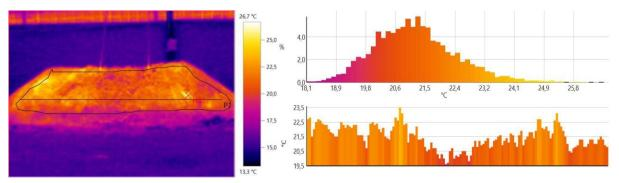
Figure 14. Static temperature field of the surface of the composting pad №1 (composting pad height of 1.5 m without further mechanical aeration and additional humidification)
