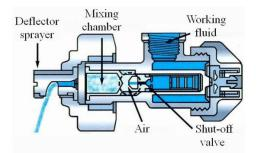
**Figure 1.** Hydropneumatic deflector AirJet nozzle (TeeJet Technologies)
