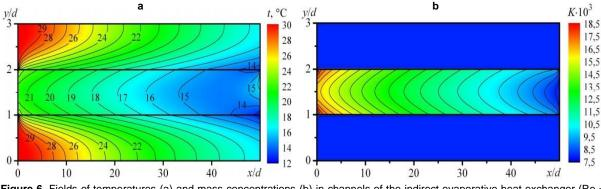
**Figure 6.** Fields of temperatures (a) and mass concentrations (b) in channels of the indirect evaporative heat exchanger (Re = 100,  $t_0 = 30$  °C,  $\phi_0 = 30$ %)
