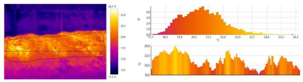
Figure 17. Static temperature field of the surface of the composting pad №4 (composting pad 1.5 m high with subsequent mechanical aeration and with additional humidification)
