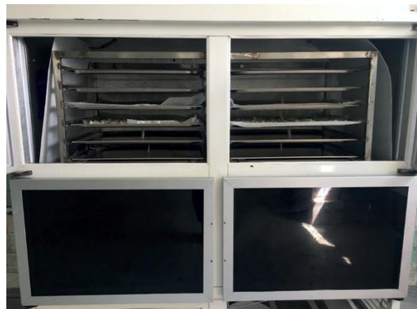
**Figure 8.** The TSU convective dryer
