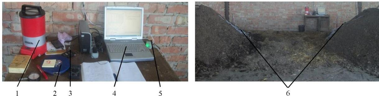
**Figure 3.** Measuring instruments and equipment (1 – moisture meter VLK-01; 2 – construction roulette; 3 – electronic manual scales; 4 – personal computer; 5 – electronic thermometer TM-32/H-5T; 6 – DS18B20 temperature sensors)
