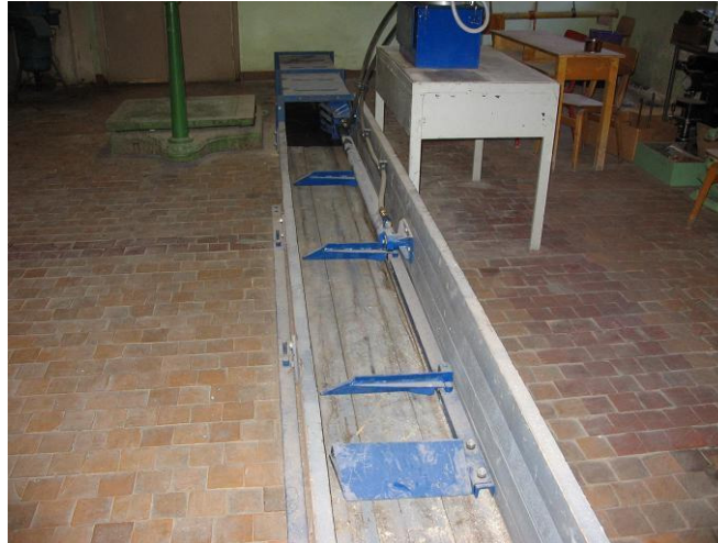
Figure 5. The device of the press manure removal, created for experiments by the idea of V. Veinla
