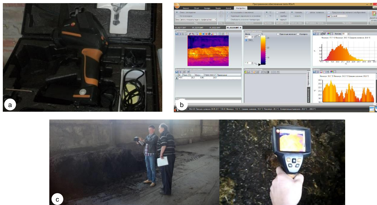
Figure 5. General view of the Testo-875 thermal imager (a), Testo IRSoft software (b) and the temperature measurement process (c)
