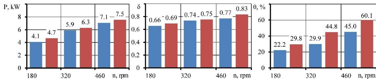
**Figure 10.** Comparisons of research results for single (blue) and double (red) working bodies that are placed on PRT-10 for cow manure
