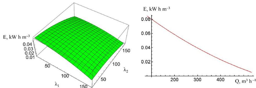
**Figure 9.** Dependence of the aerator's specific energy consumption from research factors
