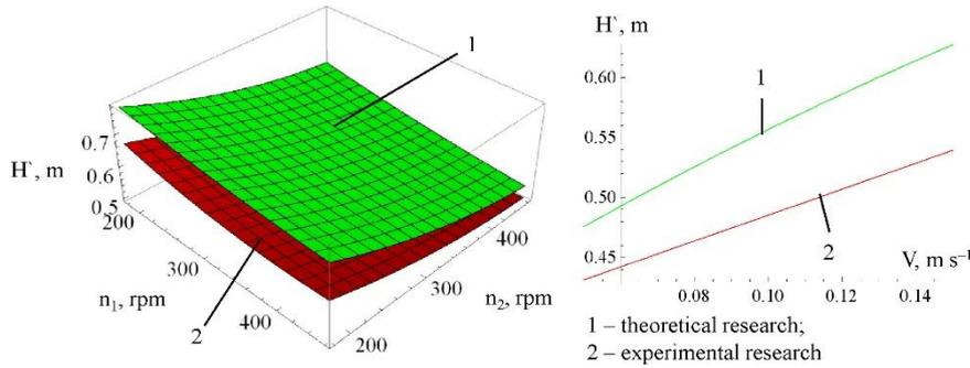
Figure 7. Dependence of the formed compost mixture height from the research factors
