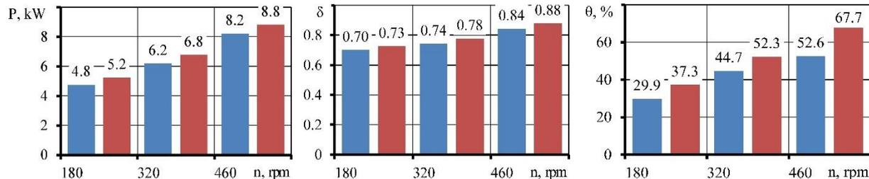
**Figure 11.** Comparisons of research results for single (blue) and double (red) working bodies that are placed on an aerator
