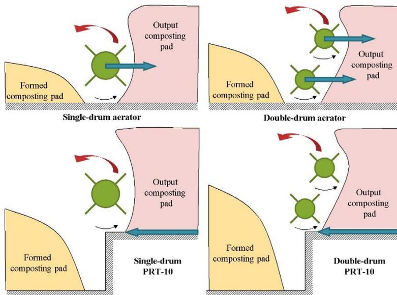
**Figure 1.** Rotary drum-blade grinding, mixing and formatting machines operation schemes
