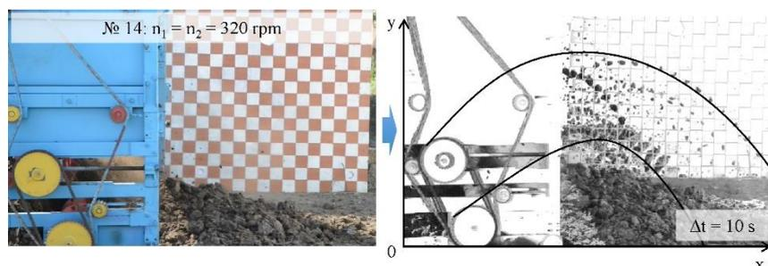
**Figure 4.** Visualization of the compost mixture particles movement process under the impact from the working bodies of the universal experimental installation
