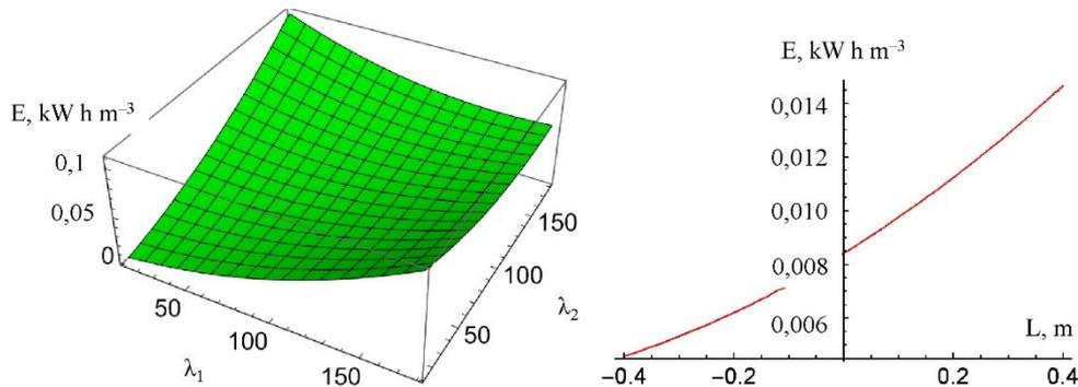
**Figure 6.** Dependence between the specific energy consumption of mechanical aeration mixing process and research factors
