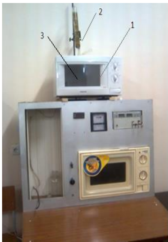
Figure 1. Photo and scheme of the experimental installation for oil extraction in a microwave field
